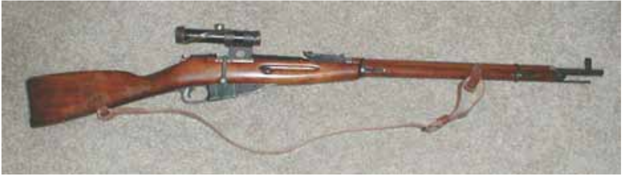
Mosin Nagant 1891/30 Sniper Rifle with a three power PU scope
